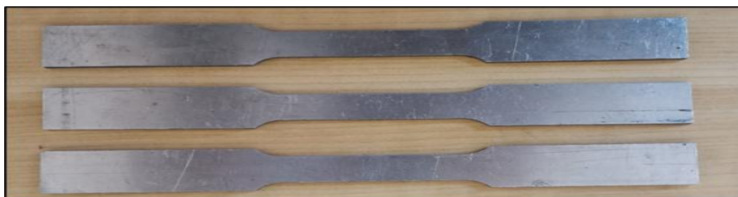
Figure 3-16: The general shape and dimensions of tensile specimens E8.
