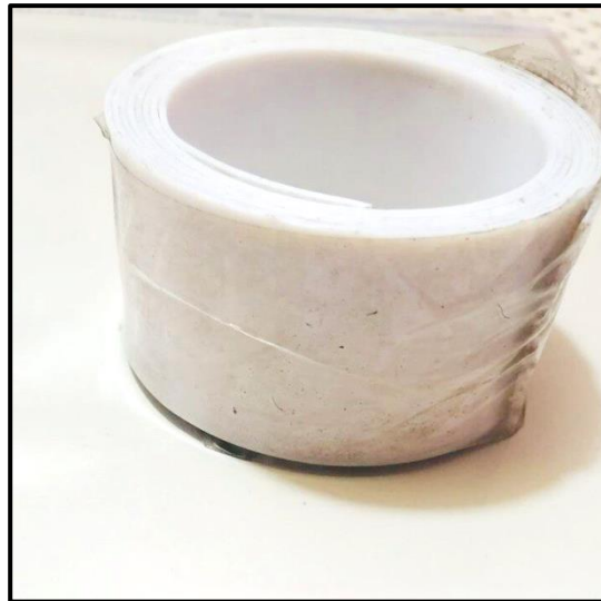
Figure (4-2): The Polytetrafluoroethylene (PTFE) ribbon used for shock absorption and to increase the flexibility of the fabricated lower limb.
