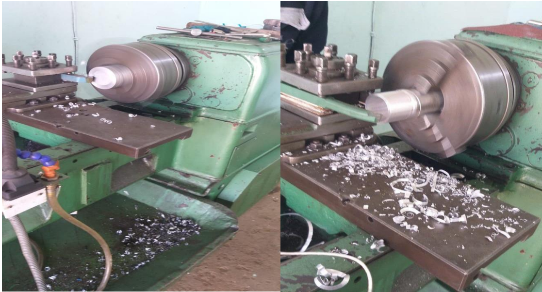
Figure (4-6): The fabricating of the below knee prosthesis limb parts using the lathe machine
