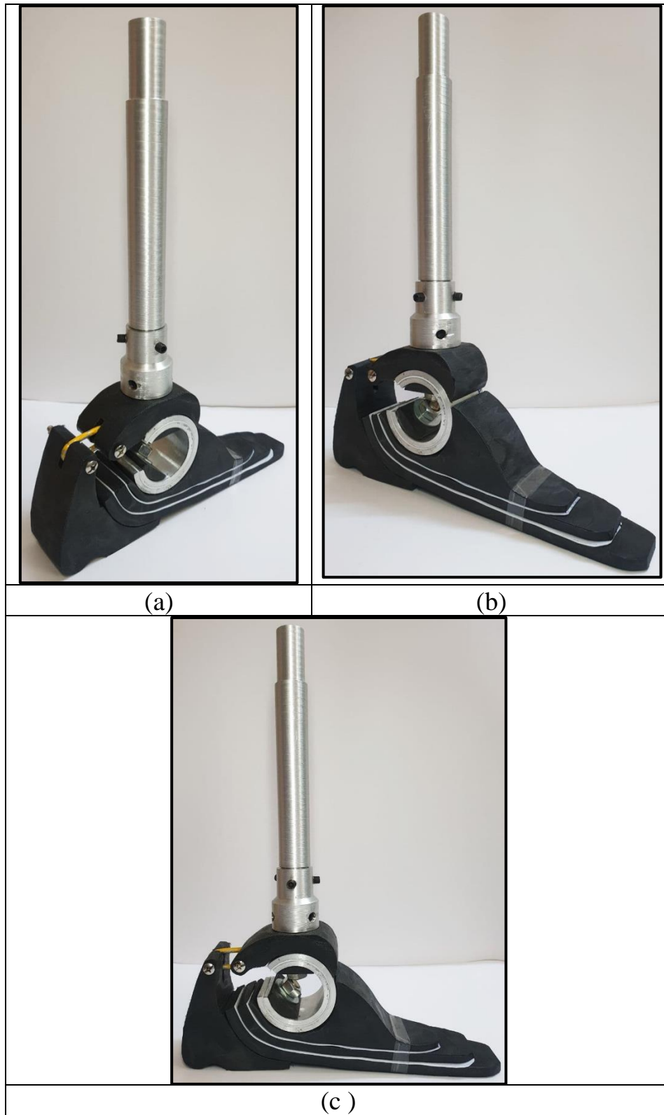
Figure (4-10): The final assembly of the prosthetic leg parts after the completion of the drilling and threading operations
